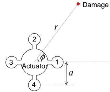
Figure 1: SHM node orientation and coordinate system
