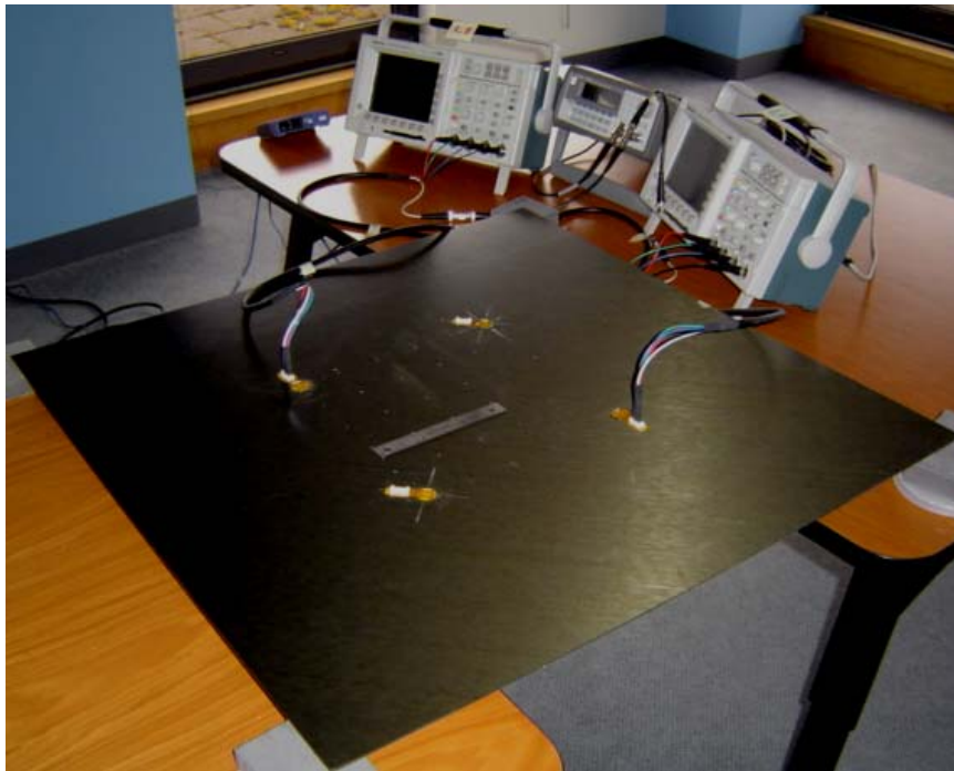
Figure 2: Photograph of experiment with “blind” composite plate and 4 SHM nodes
