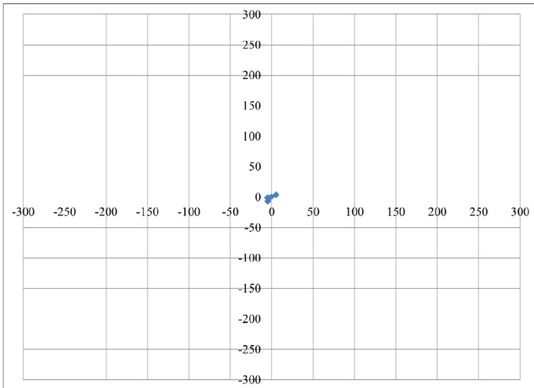
Figure 5: Active GW fastener detection results, re-centered to a common origin. Mean error ~ 5 mm
