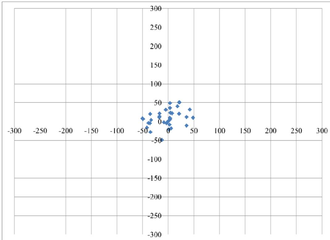
Figure 3: Passive AE impact detection results, re-centered to a common origin. Mean error ~ 25 mm
