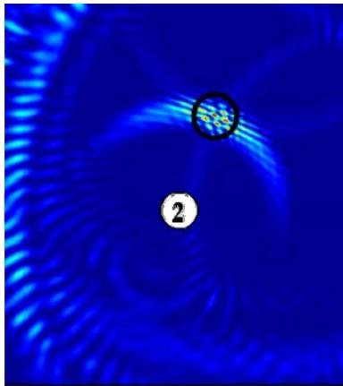
Figure 2: Phase coherent imaging on an aluminum plate with a magnet target
