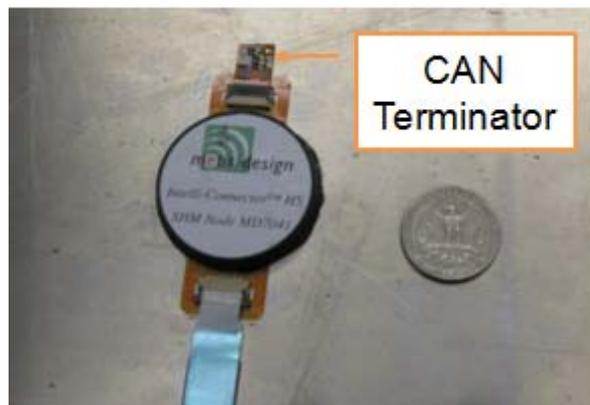
Figure 1: Digital node and analog sensor based bonded an aluminum plate with FFC attached
