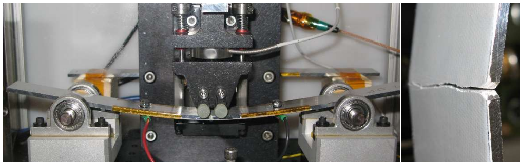
Figure 6: Photograph of 4-pt fatigue bend fixture (left) and fatigue crack growth (right)
