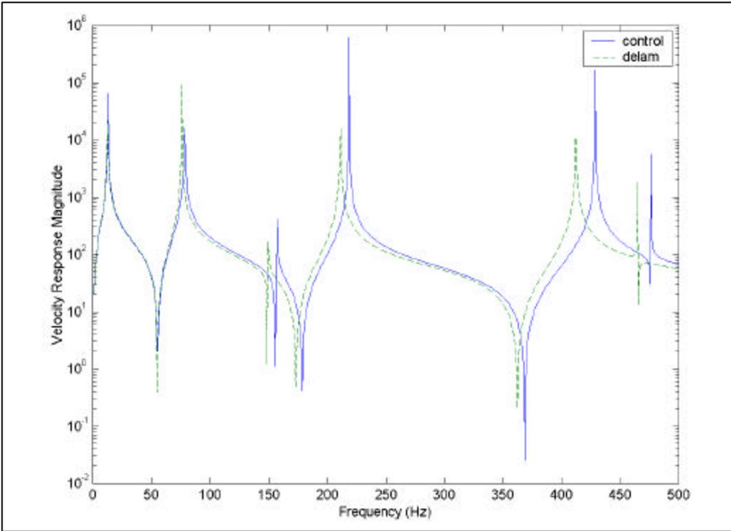
**Figure 3:** Frequency response transfer function plot from I-DEAS, range of 0-500 Hz
