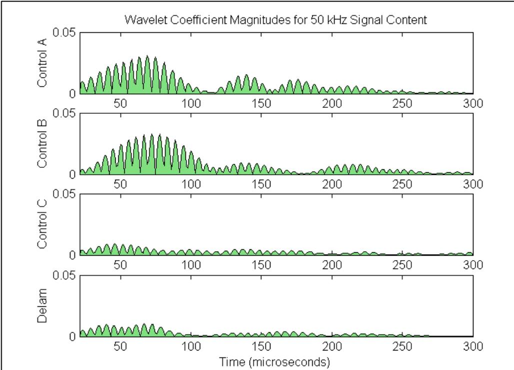
**Figure 4:** Wavelet coefficients for beam “blind test”; compares 50 kHz energy content for control beam specimen and 2 specimen with delamination
