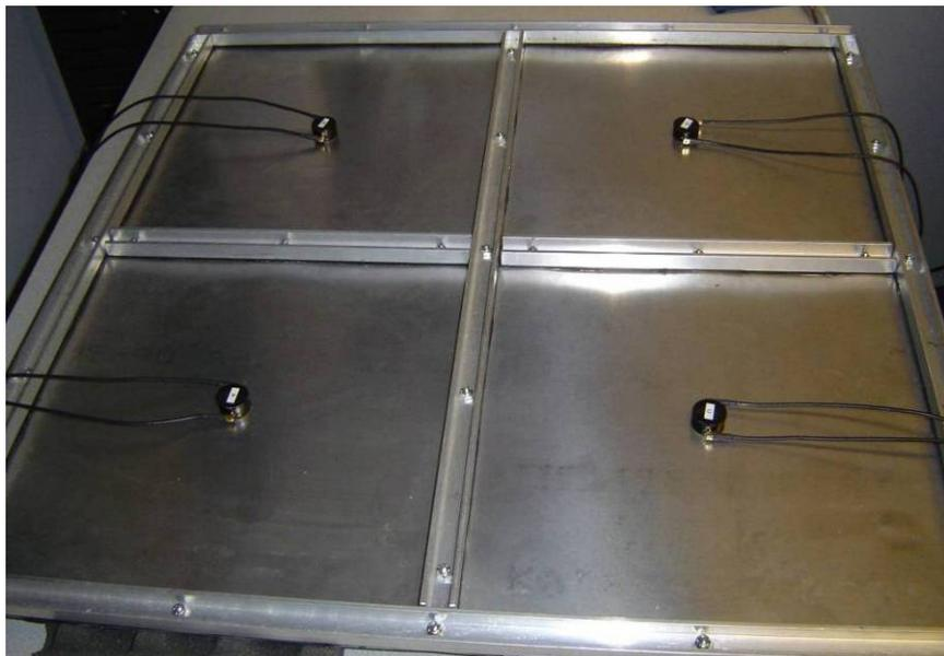
**Figure 2:** Photograph of representative aircraft testbed with M.E.T.I.-Disk 2 sensors attached.
