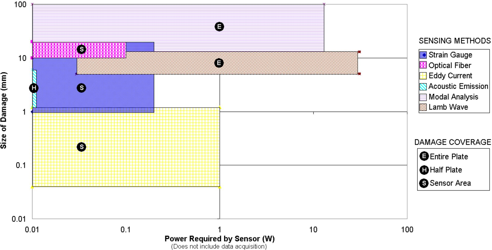
*Methods with lowest power requirement typically have lowest coverage; Lamb wave and FR: sensitivity scales with power level*
