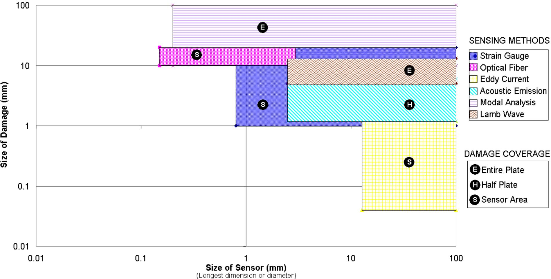
*Trade off between damage detection size and coverage
