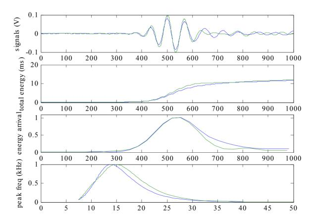
• Some matrix cracking caused a slight time delay, less tail energy and a small shift to a higher frequency bandwidth
