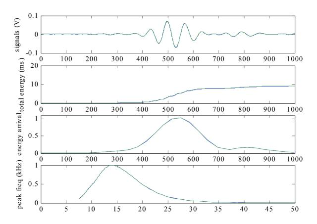
Highly reproducible signal between same set of actuators and sensors tested several times
