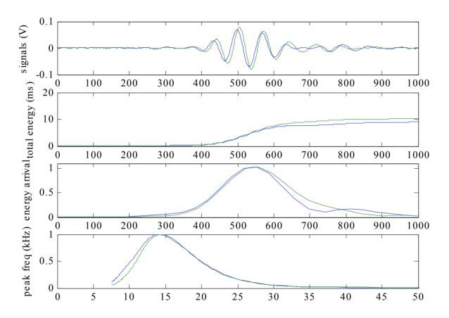
Similar response between pairs of actuators/sensors located on several undamaged plates
