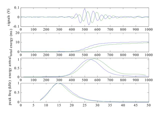
• Delaminated signal is time-lagged, and has slightly lower energy content. Frequency bandwidth remains similar
