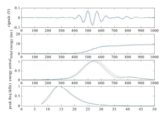
Similar response across several different pairs of equally spaced actuators/sensors on same plate
