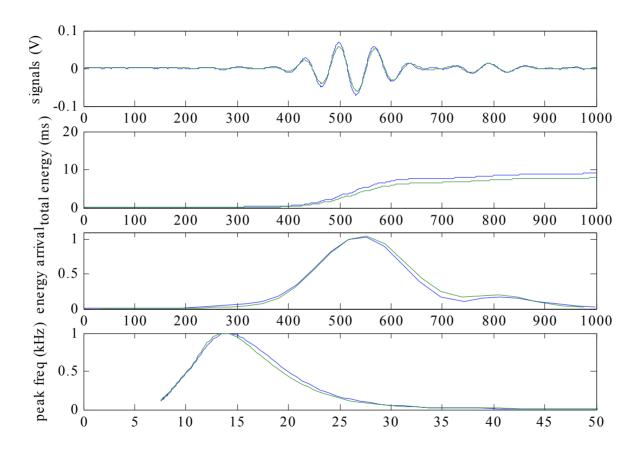
Signal shape remains unchanged when propagating in reverse direction, other metrics remain similar
