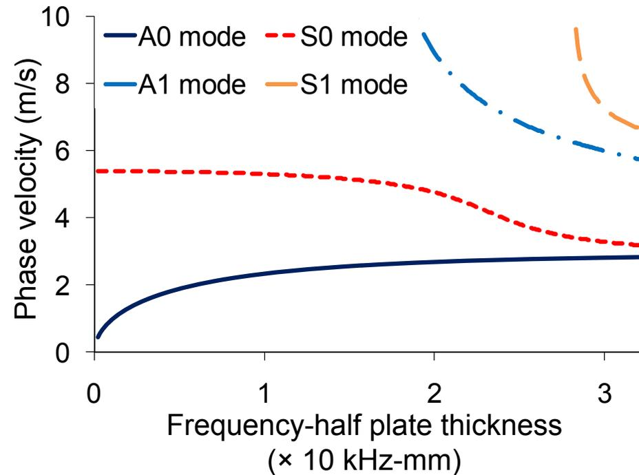
*Phase speed dispersion curve for aluminum plates*
