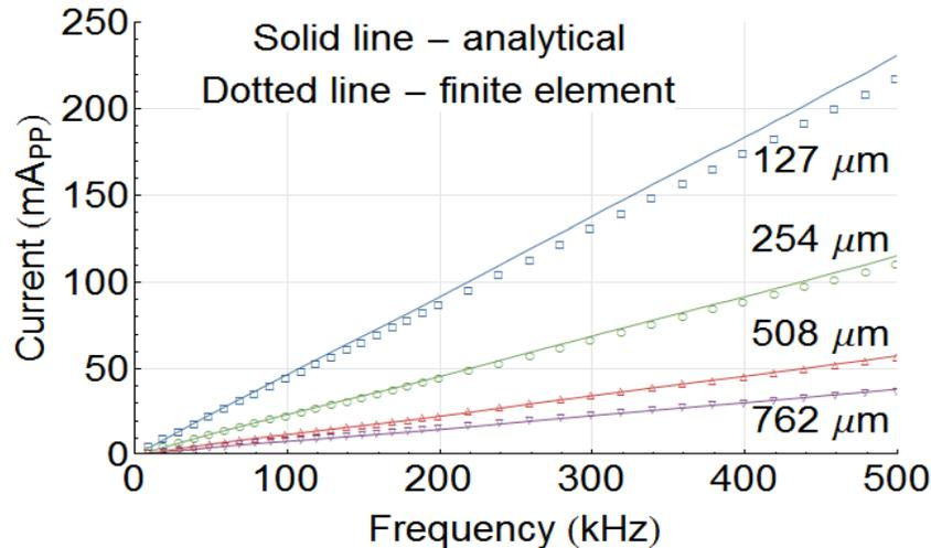
*Current versus center frequency for various thickness actuators*
