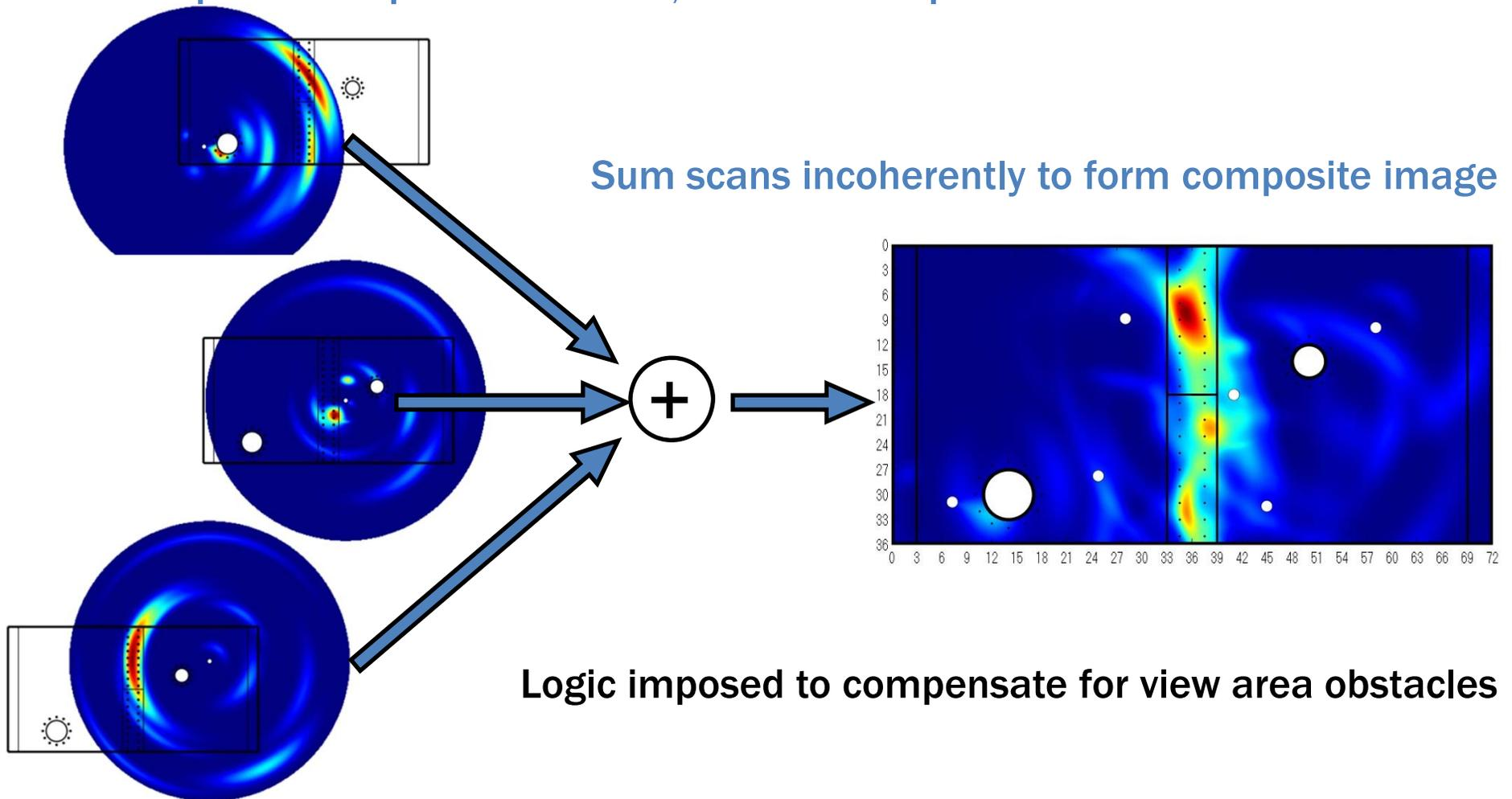
color represents # of standard deviations above mean of damage-free data
