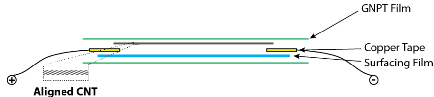
Figure 1: Side view of aligned CNT film resistive heater and cure status sensor.
