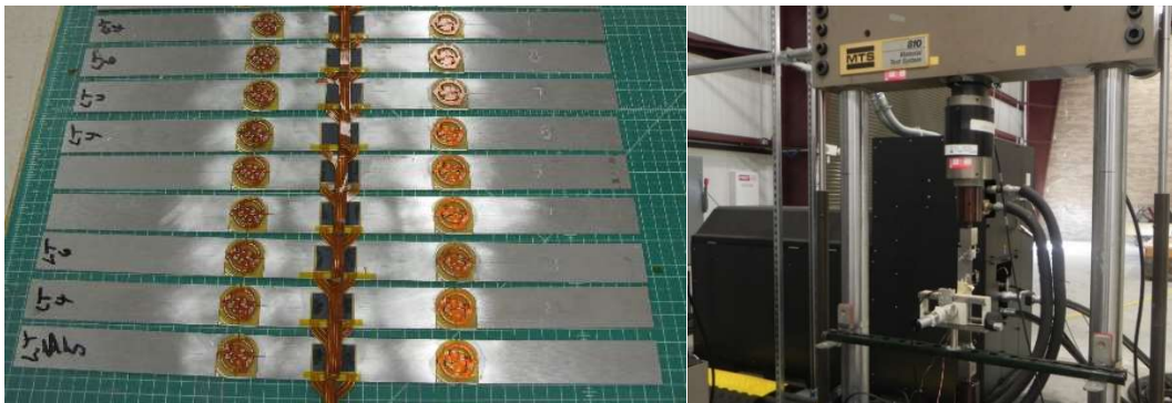
Figure 6. Al-Li tensile-tensile fatigue specimens instrumented with ultrasonic PZT arrays (left). MTS setup for fatigue crack growth and optical measurement of actual crack length (right)
