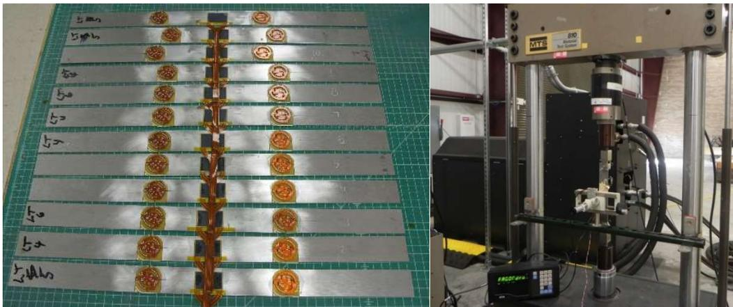
Figure 7. Al-Li tensile-fatigue specimens instrumented with CNT crack gauges (left). MTS setup for fatigue crack growth and optical measurement of actual crack length (right)
