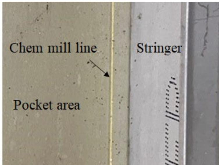
Figure 1. FASTER panel chemical mill line
