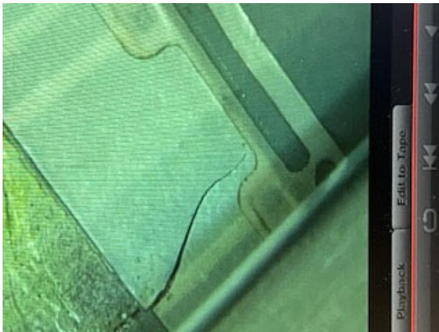
Figure 5. Crack through Metis Design sensor
