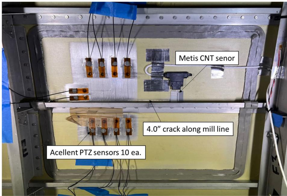
Figure 2. Sensor layout on both sides of 4" sawcut
