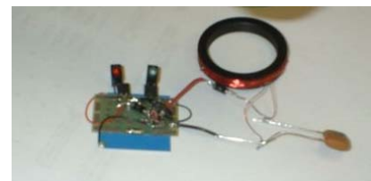
Inductive loop recharger
